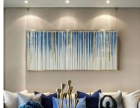
Directional downlights to illuminate artwork
