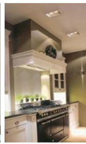
Bulkhead above kitchen island with linear LED around to uplight the ceiling. Downlights for task lighting. Linear LED concealed in the skirting board.
